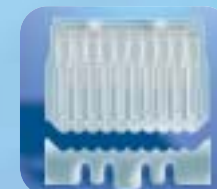
4 th step The pre-moulded receptacle is filled, then the upper part is moulded and sealed
